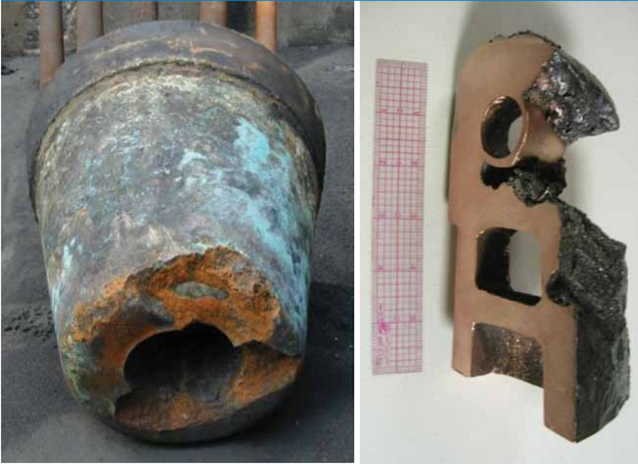
Two tuyeres from different operations, both dual-chamber style with a cast-in copper pipe.
