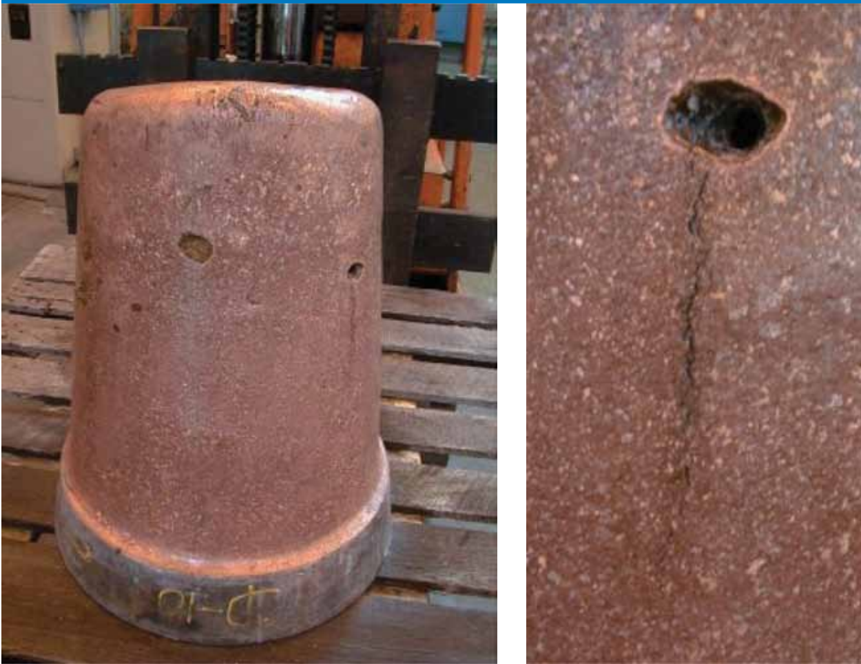
Typical tuyere failure, with tuyere cleaned and etched to reveal defects and grain structure.
