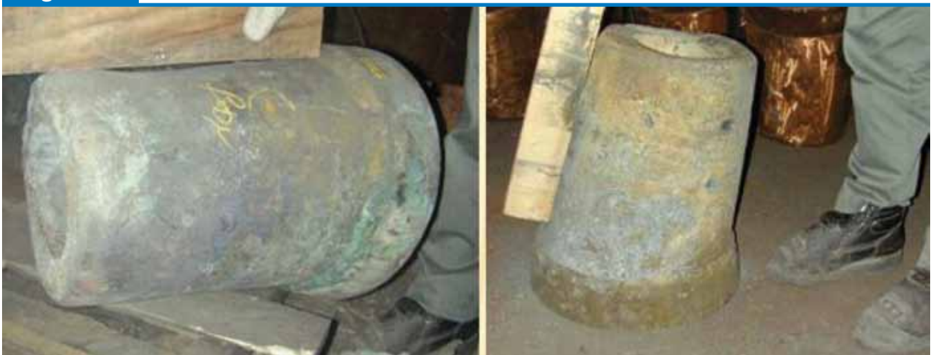
Failed tuyere (left) made of bare copper, and a used tuyere (right) that was calorized.
