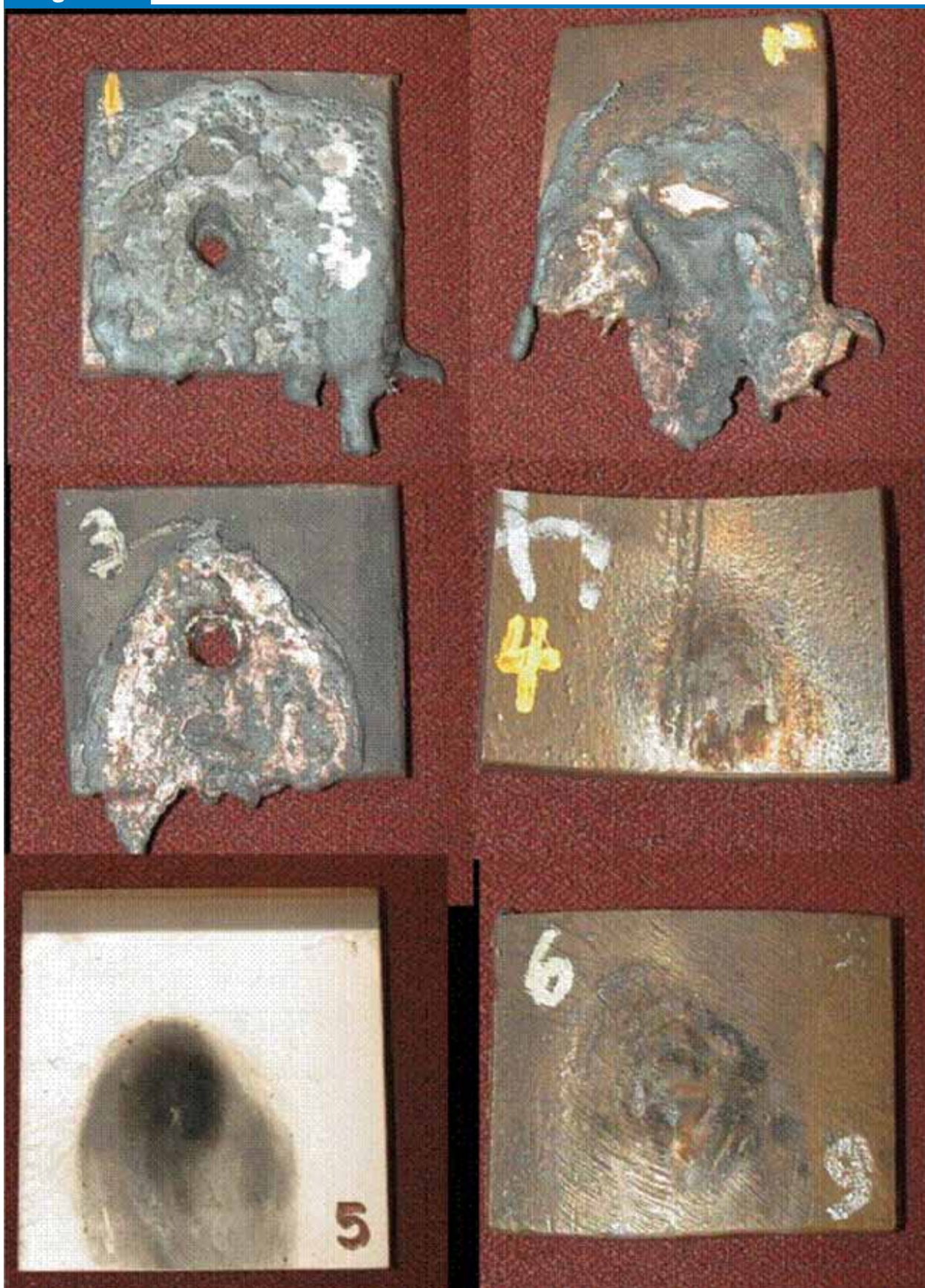
Results of splash testing. Samples 1 and 3 = bare copper; sample 5 = ceramic coated copper; samples 2, 4 and 6 = calorized copper.
