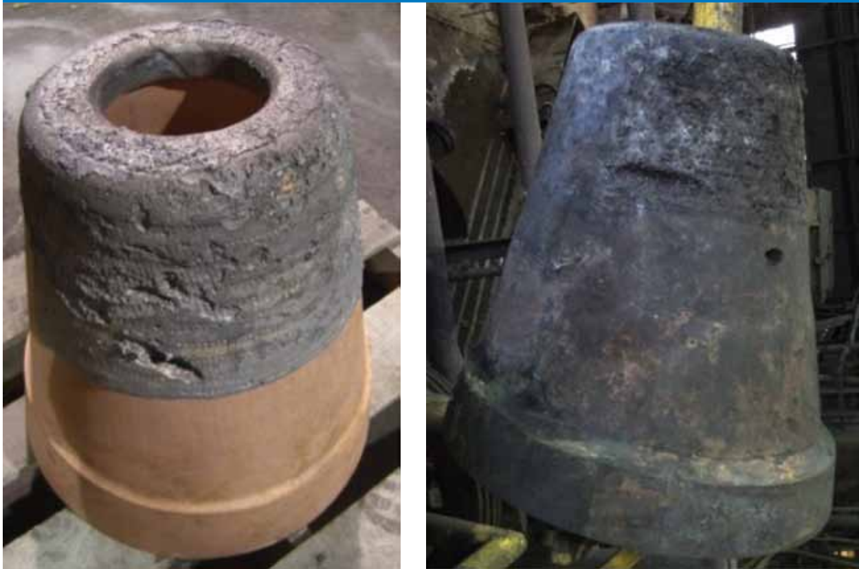
Two tuyeres that failed through the hard-surface welds: (a) sandblasted and (b) as removed.
