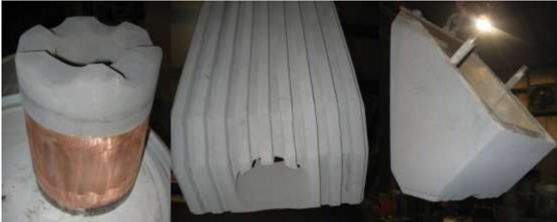
Figure 10. Calorized copper EAF castings. Burner (left) and burner panel (center & right) currently undergoing trials.
