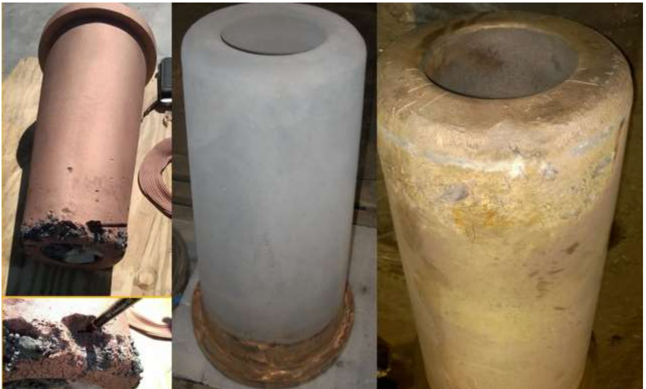
Figure 8. Cupola tuyere failure due to liquid iron penetration (left), new tuyere as calorized (center) and removed from service and sandblasted for inspection (right), absent iron penetration.
