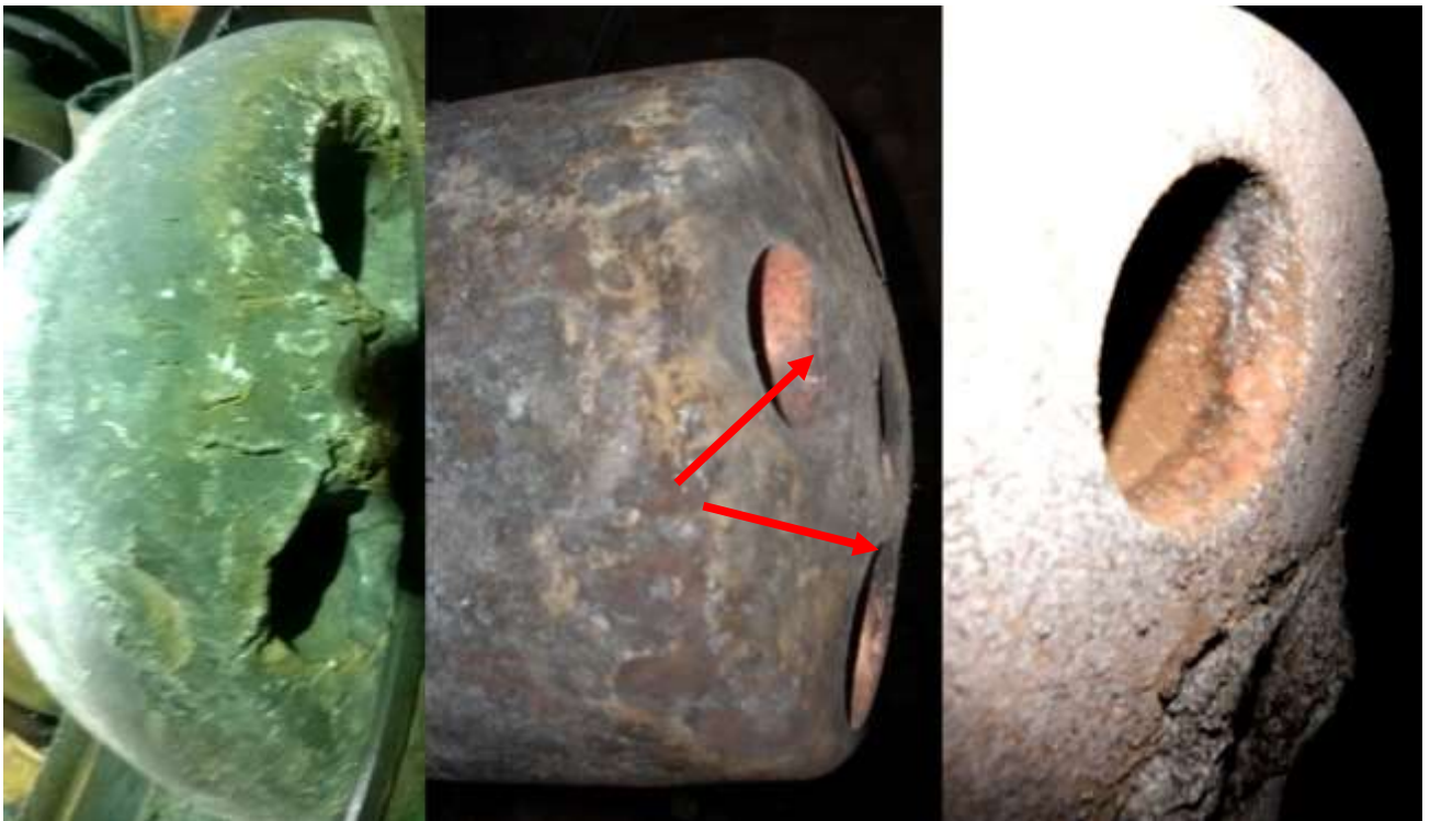
Figure 9. Typical failed BOF lance tip with major port wear (left), uncalorized lance with port wear at 99 heats, and calorized lance with no port wear inspected at 96 heats.
