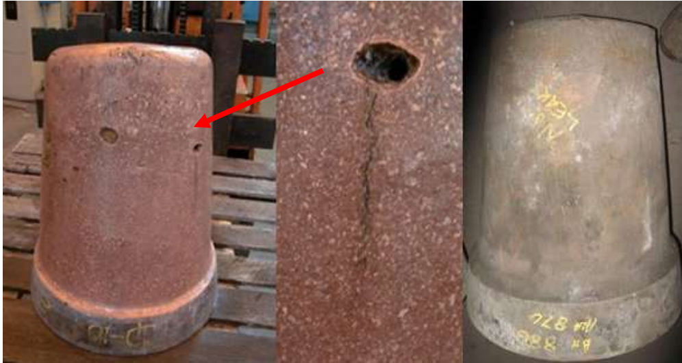
Figure 7. Typical plain copper tuyere failure (left and center), with tuyere cleaned and etched to reveal defects and grain structure, vs. calorized tuyere changed for age at 1,317 days, no leaks, no burns, same furnace (right).
