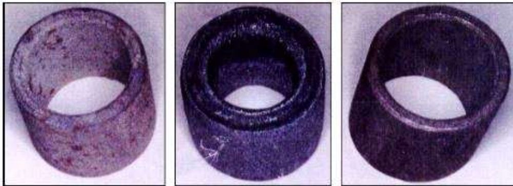
Figure 3. Samples of calorized, uncalorized, and control pipe (steel) subjected to oxidation testing.
