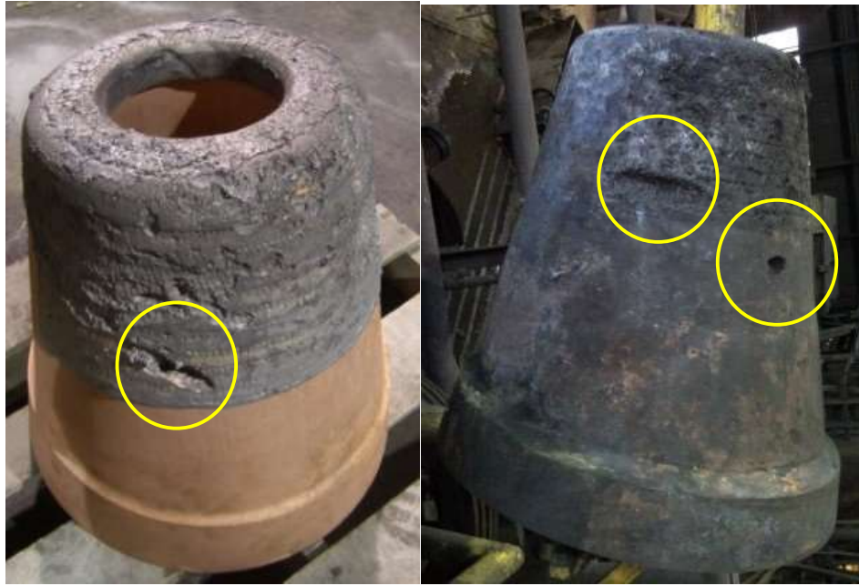
Figure 12. Two different tuyeres, failed at the hard-surface welds. Sandblasted (left), as removed (right)
