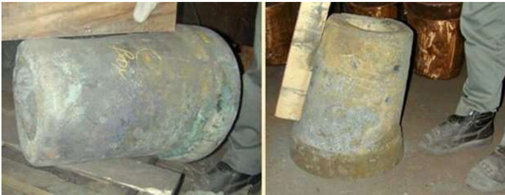
Figure 11. Worn, failed tuyere (left) bare copper 685 days, calorized tuyere (right), 774 days.
