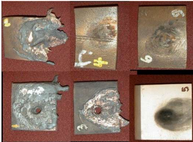
Figure 6. Lab results of splash testing: samples 1 and 3 - bare copper; sample 5 - ceramic coated copper; samples 2, 4, and 6 – calorized copper.
